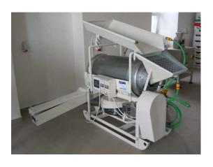
Urga's trommel centrifuge concentrator device is used to classify and subsequently to gravitationally concentrate granular materials. This applies especially to alluvial placer raw materials, with possible content of clay, or to pulverized ore material.
